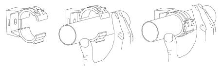
Simply mount CLIC, push pipe in by hand, grips and locks by applying slight pressure. To open: unlock the CLIC latch with screwdriver.
